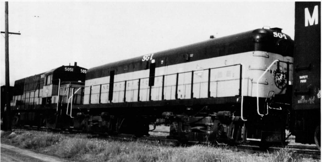
The Milwaukee slug SG1, in company with a number of U25Bs and U28Bs, was among the various pieces of equipment gathered up for the eastward trek. The SG1 Slug was a cut-down Alco RS unit that received electricity for its traction motors from a powered unit. Its last assignment was working the Tacoma Hill, adding its effort to move freight.
